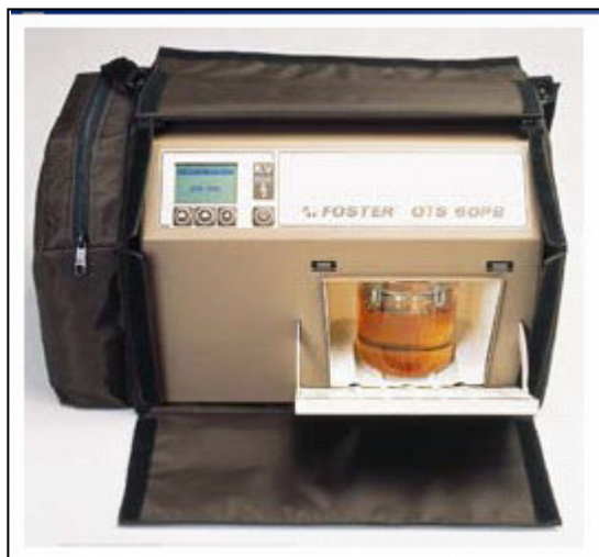
Fig.1 Measurement of oil breakdown voltage by testing equipment Megger
